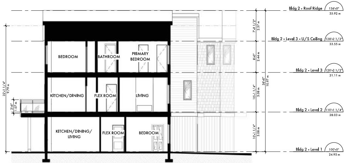
2 Building 2 - East-West Section Looking North Scale: 1 : 75
