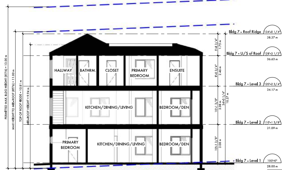
4 Building 7 - North-South Section Scale: 1 : 75
