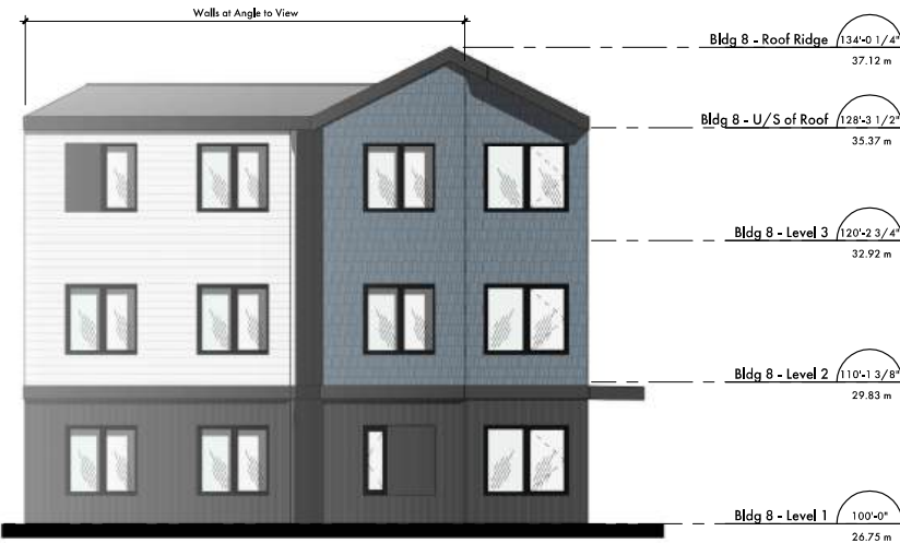
Building 8 - West Elevation Scale: 1 : 75
