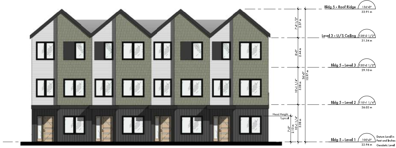
Building 5 South Elevation Scale: 1 : 75
