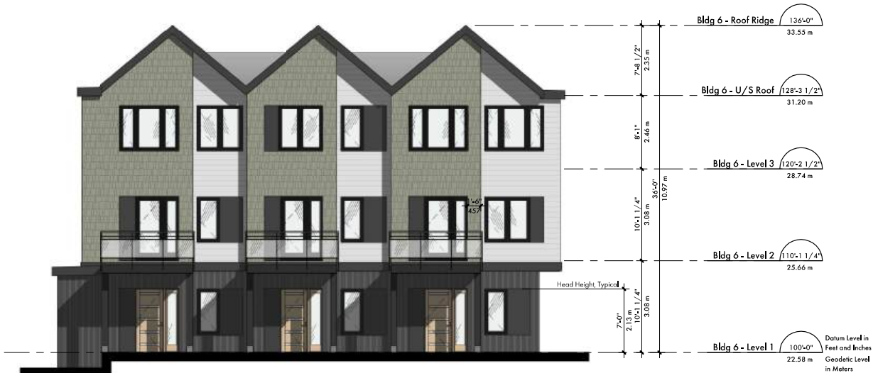
Building 6 North Elevation Scale: 1 : 75
