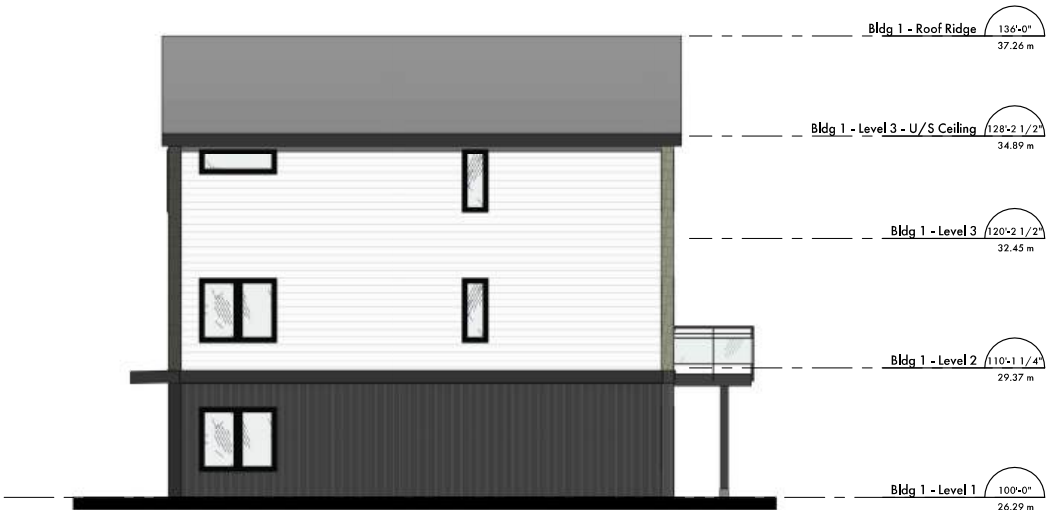
Building 1 - North Elevation Scale: 1 : 75
