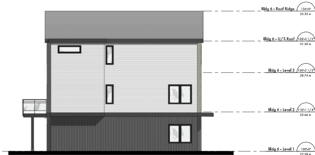
Building 6 - West Elevation Scale: 1 : 75
