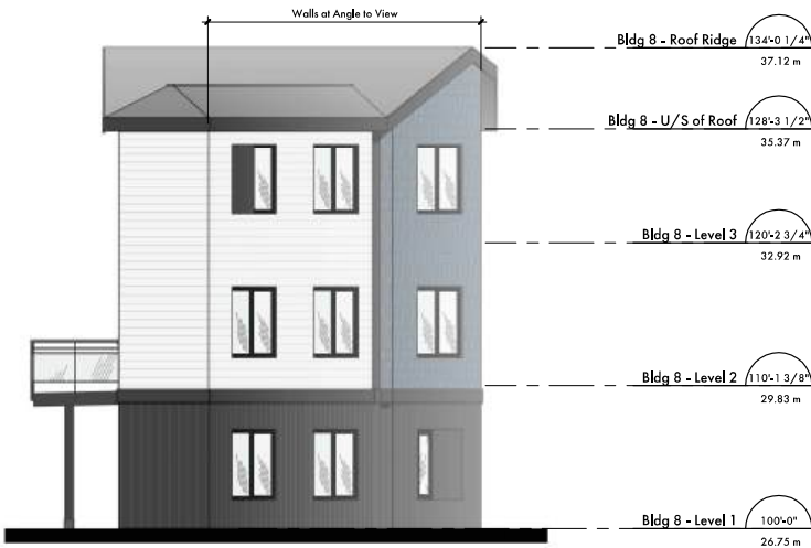
Building 8 - North Elevation Scale: 1 : 75
