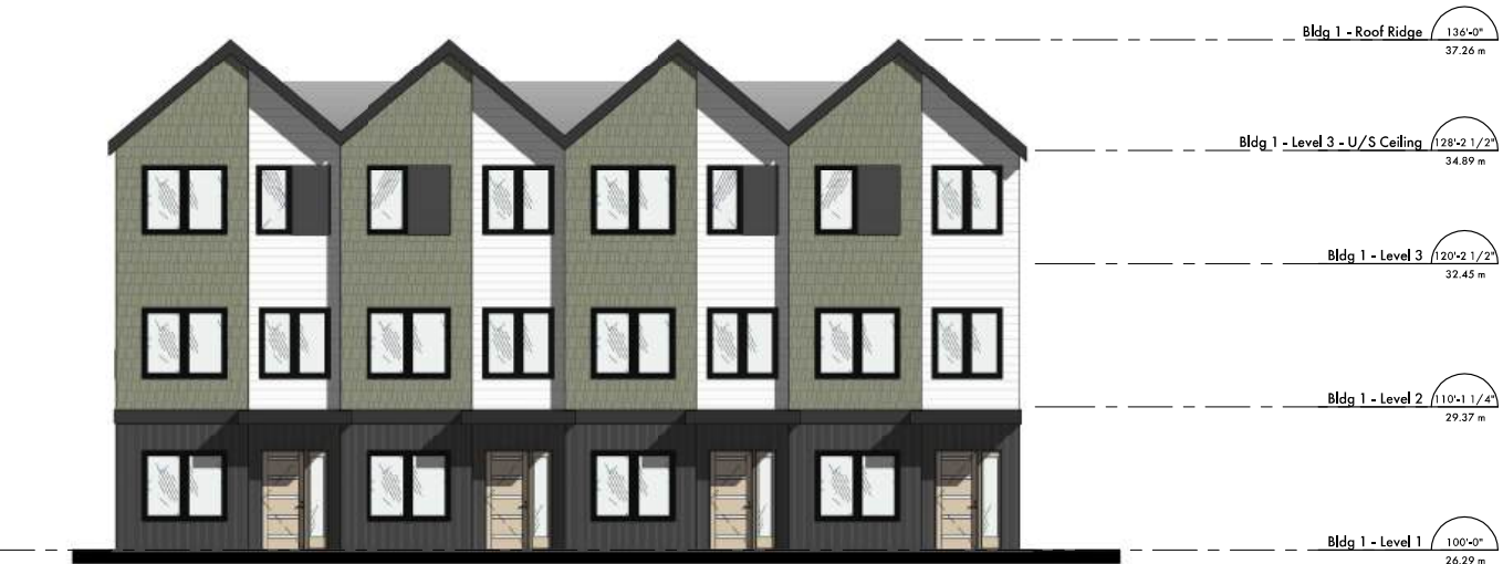
Building 1 - East Elevation Scale: 1 : 75
